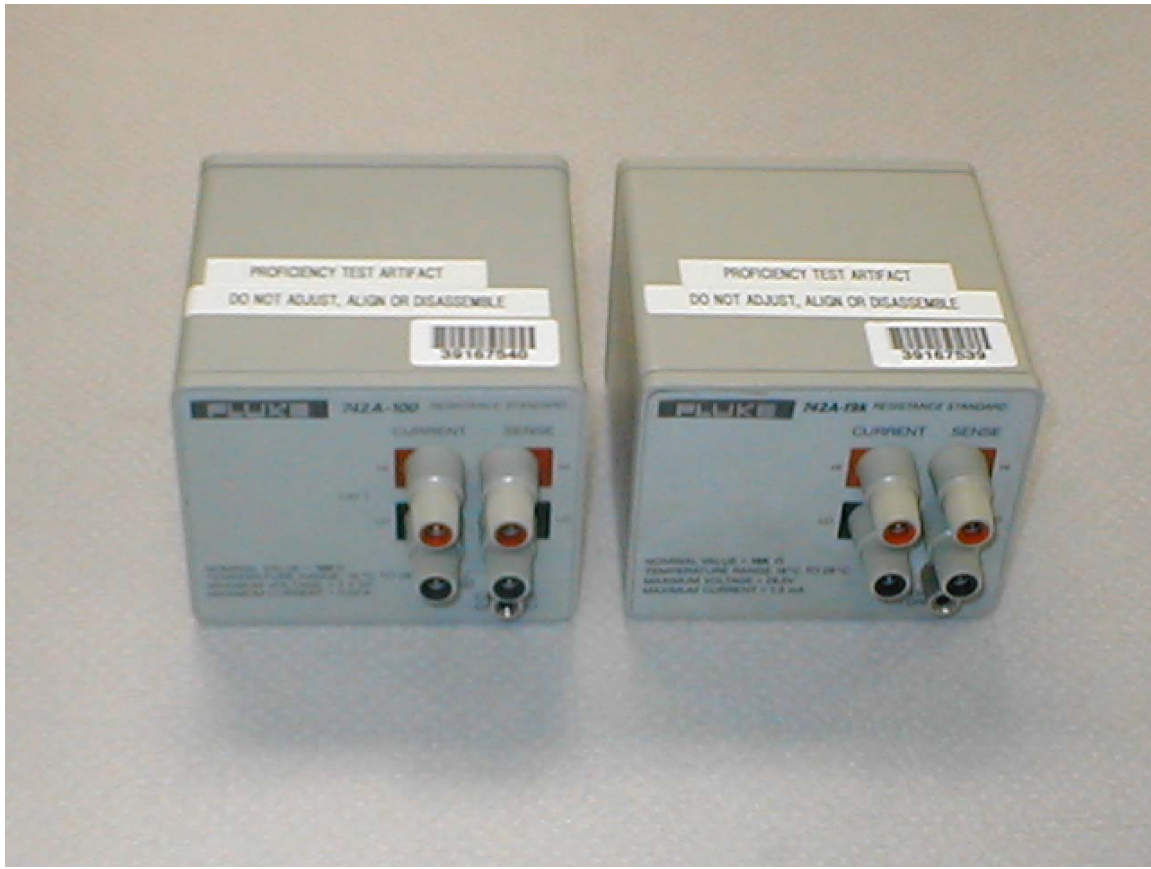
Figure 1, Fluke 742A 100 ohm and 19 kohm Standard Resistors
