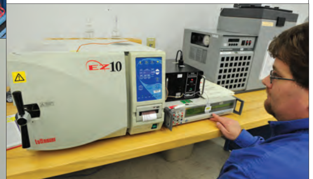
Autoclave repair and calibration
