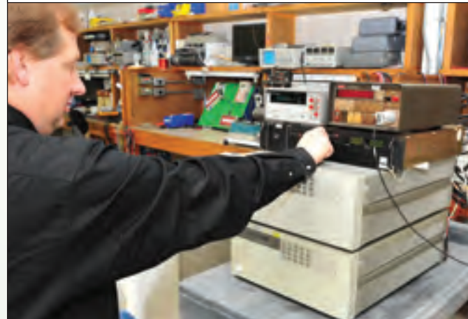
High voltage power supply repair and calibration
