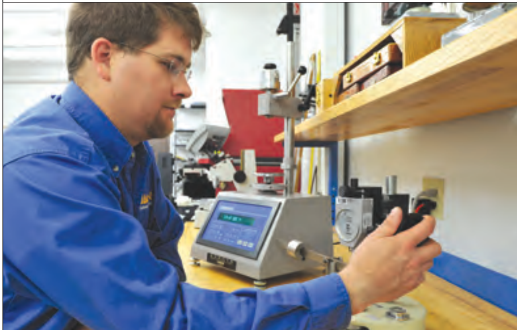
Calibration of durometer force and durometer tip dimensions
